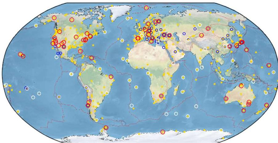
**Global space-geodetic network used to determine JTRF2014. Gold dots are GNSS sites (671); Red circles are VLBI (71); Blue circles are SLR sites (71); White circles are DORIS sites (159). Polygons in red represent tectonic plate boundaries.**
